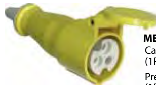
MESV110 Cable mount plug: 16A 110-130V AC (1P+N+G), protection (IP44). Spina volante diritta: 16A 110-130V AC (1P+N+T), protezione (IP44).
